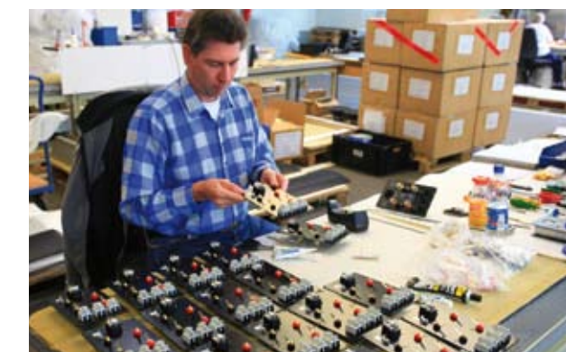
Solitaire terminals: top quality switches and sockets being assembled by hand.
