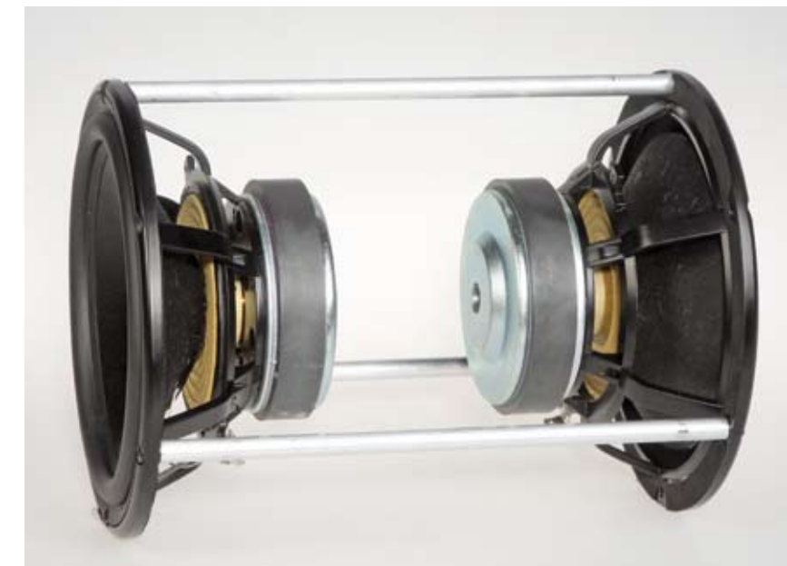
Connected: Pairs of bass drivers are screwed together via rods and oscillate conversely. Any structure-borne sound is thus almost completely eliminated.
