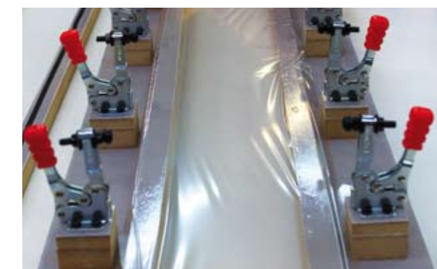
The foil diaphragm is only five micrometres thick, seen here not yet pulled taut.
