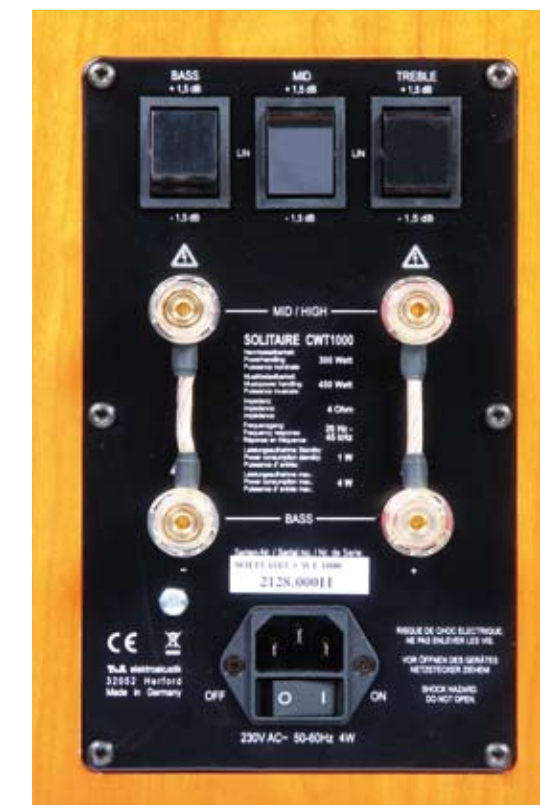
The terminal: top the switches for adjusting the speaker to the room. They only have a subtle (mid-range) or narrowband (bass and treble) effect. The connectors are all designed for bi-amping. The mains supply is used only for the electrostatic speaker's constant polarization voltage.
