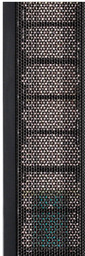
Behind bars: the wafer-thin foil oscillates between two electrically pre-charged stator grids. Reinforcements and protective circuits appear through the grid only on this photo.
